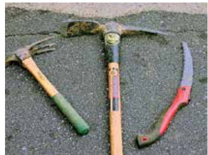
Manual tools for kudzu root crown extraction.
