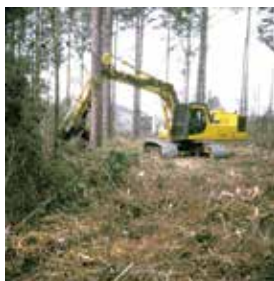
Boom-mounted mulcher head.
