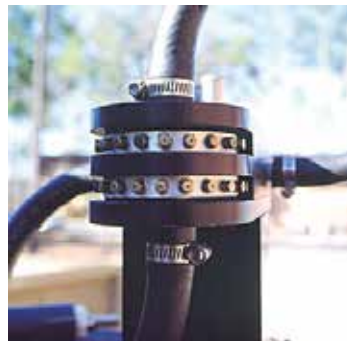
Radiarc ® Sprayer 22-tip head.
