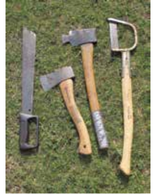
Cutting tools for hack-and-squirt treatment.
