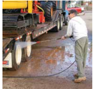
Clean seeds and plants from equipment with pressure washer.
