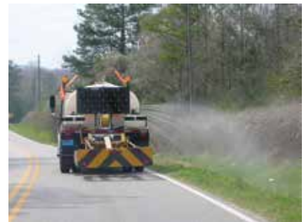
Roadside sprayers can treat invasives along highways.
