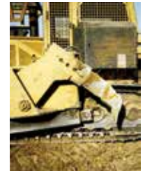
Ripper shank on bulldozer in the up position.
