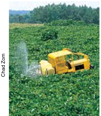
Boom Jet® nozzle on a crawler tractor spraying kudzu.
