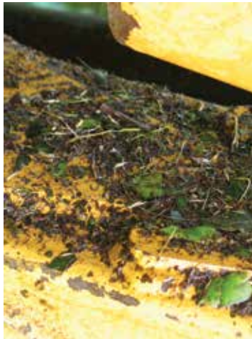
Excess grease traps seeds.
