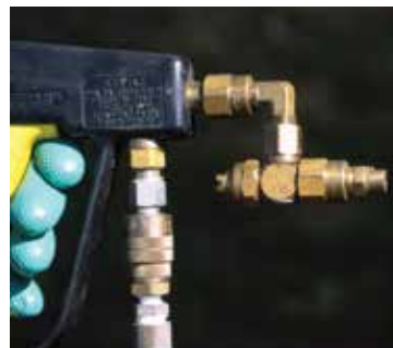
Spray gun with rollover valve that holds two tips.
