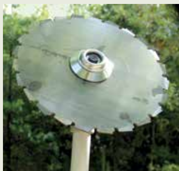
Brushsaw blade with chainsaw-like teeth.
