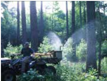
RTV mounted sprayer with Boom-Buster nozzles.
