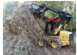
Skidloader uprooting kudzu vines for removal.
