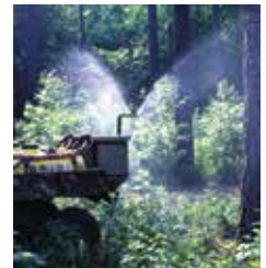
Spray pattern of two Boom Buster nozzles.
