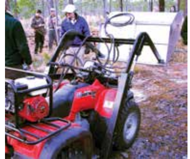
Grass seed harvester on an ATV.
